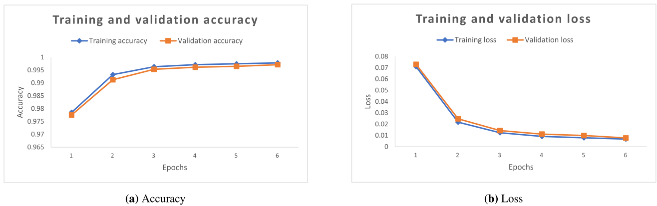
FIGURE 6 Training and validation performance of the proposed self-attention convolutional neural network on X-IIoTID dataset.
