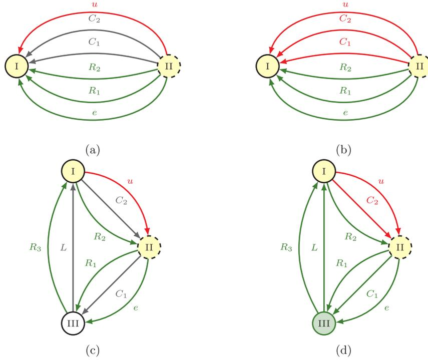
Fig. 6.2. Wind turbine models as linear graphs. Yellow nodes are shared and the dashed node is ground. (a) and (c) Initial graphs for one- and two-inertia models, respectively. (b) and (d) Graph-splitting decompositions for one- and two-inertia models, respectively.
