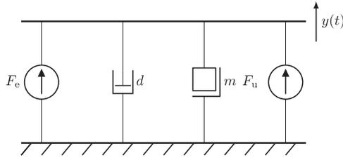
Fig. 4.1. Mechanical system diagram of the damped mass.
