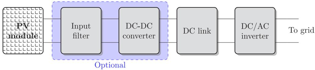
Fig. 5.1. Schematic of grid-connected PV system.
