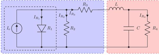
Fig. 5.2. Electrical circuit model for PV solar cell (blue box) and RLC filter (red box). The components inside the black box comprise the ideal PV cell.
