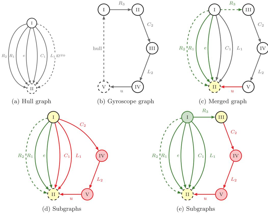
Fig. 7.1. Linear graphs for wave energy converter with linearised coupling. Dashed green edges are absent when corresponding damping term is omitted, and present otherwise. Yellow nodes are shared and the dashed node is ground. (a) Hull graph (with mobility analogy) (b) Gyroscope graph (with impedance analogy) (c) Merged wave energy converter graph. (d) and (e) Subgraph and complement for undamped and damped gyroscope, respectively.
