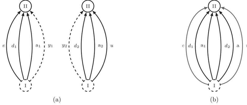
Fig. 3.2. Two rotating shafts connected by gear-train under mobility analogy. Dashed node is ground. (a) Separate graphs with dashed transformer edges (b) Merged graphs.
