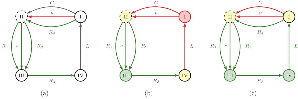
Fig. 5.3. PV RLC circuit model as graph. Yellow nodes are shared and the dashed node is ground. (a) Initial colouring of graph with RLC filter (b) Subgraph and its complement for the LC filter (c) Subgraph and its complement for the RLC filter.
