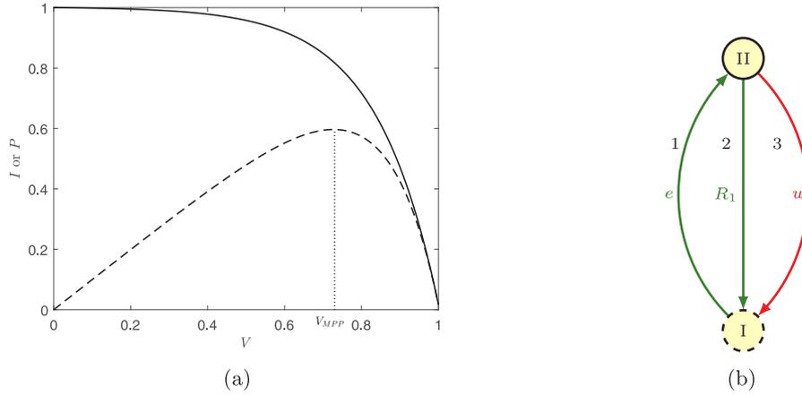
Fig. 5.4. (a)  $I-V$  characteristic (solid) and  $P-V$  characteristic (dashed) of the ideal PV solar cell. The maximum power point (MPP) is shown. (b) Linear graph for the ideal PV solar cell. The subgraph and its complement are shown. Yellow nodes are shared and the dashed node is ground.
