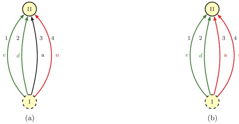
Fig. 4.2. Damped mass graph under mobility analogy. Yellow nodes are shared and the dashed node is ground. (a) Initial graph (b) Graph-splitting decomposition.
