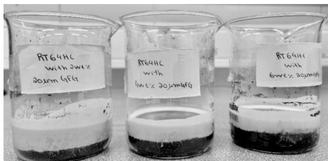
Fig. 10. Particle separation of RT64HC with mass fractions of 2, 4 and 6 wt% of 20 \mu\text{m} EG.
