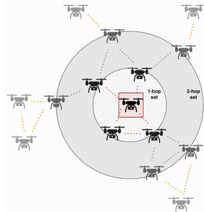
FIGURE 1. One-hop and two-hop neighboring sets from a single drone's perspective in an ad hoc network, ignoring others.
