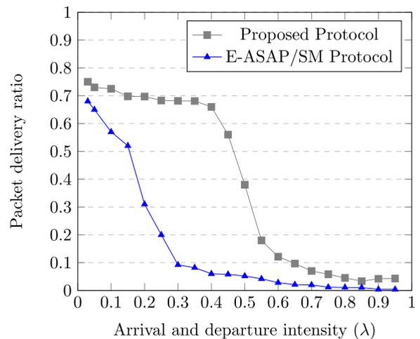
**FIGURE 10.** Packet delivery ratio performance under varying arrival/departure intensities [21].
