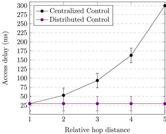
FIGURE 5. Access delay measurement under two different control strategies.
