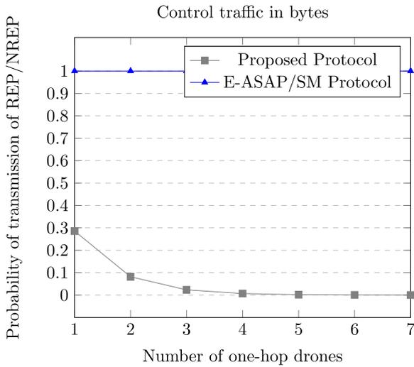
FIGURE 14. Comparison of Reply Packet (REP/NREP) transmission probabilities for the Proposed Protocol and the E-ASAP/SM Protocol during a single drone’s entry sequence. The frame size is configured to eight slots, with each one-hop drone connecting to only one further node and each node taking only one slot.
