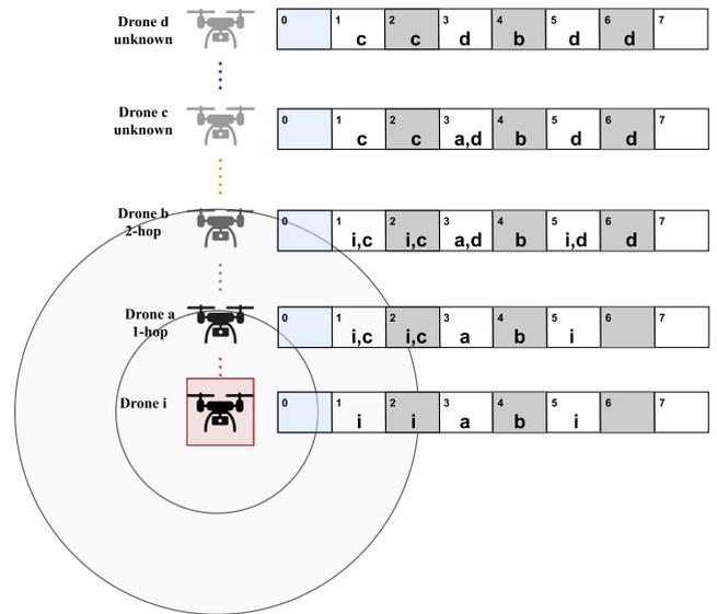
FIGURE 7. Illustration of slot reuse in a line topology.
