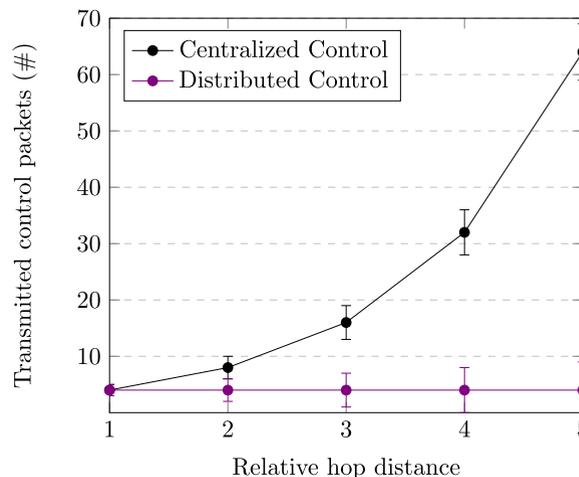
FIGURE 4. Number of transmitted packets measurement under two different control strategies.
