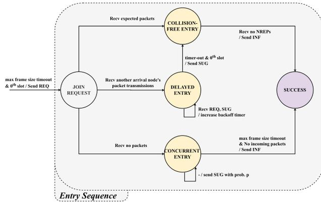
FIGURE 6. Finite State Machine (FSM) illustrating entry sequences.
