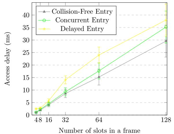
**FIGURE 9.** Access delay for different entry scenarios.
