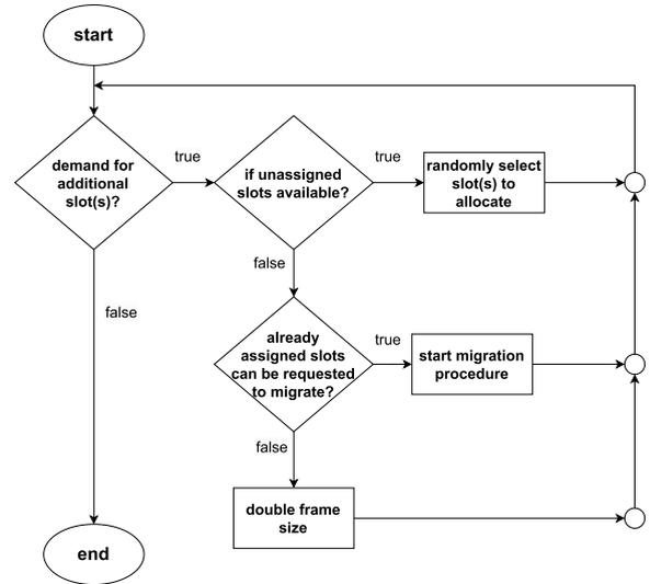
**FIGURE 8. Additional slot allocation procedure based on node's demand.**
