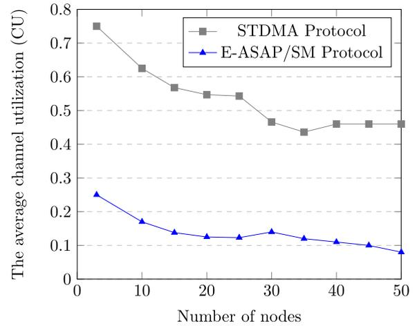
FIGURE 12. Comparison of average channel utilization achieved by E-ASAP protocol/SM and proposed protocol (STDMA) as the number of drones increases.
