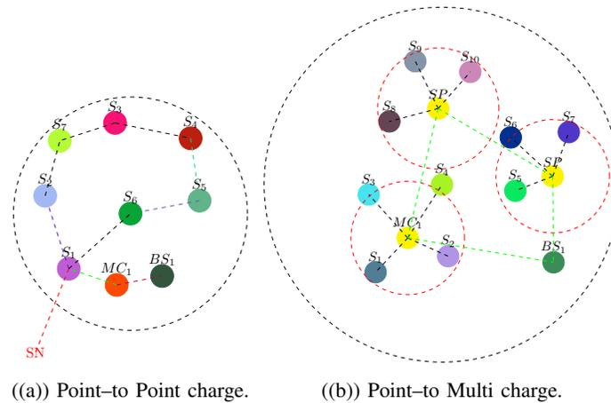
Fig. 6: Classification of The Charging Model: a) Point-to Point charge b) Point-to Multi charge.
