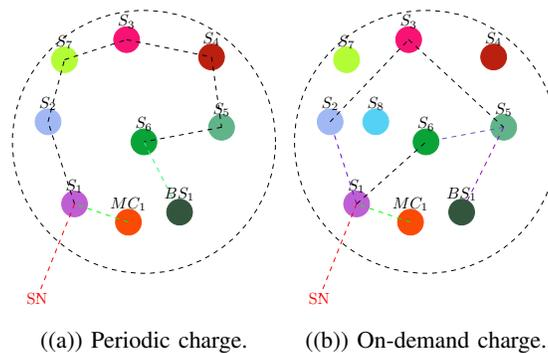
Fig. 8: Classification of the Charging Cycle: a) Periodic charge, and b) On-demand charge.
