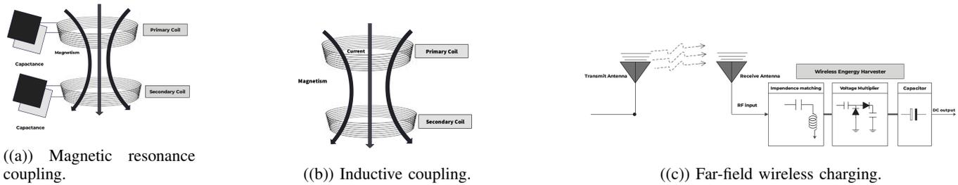
Fig. 3: Classifications of Non-radiative Coupling-based technology in WPT.
