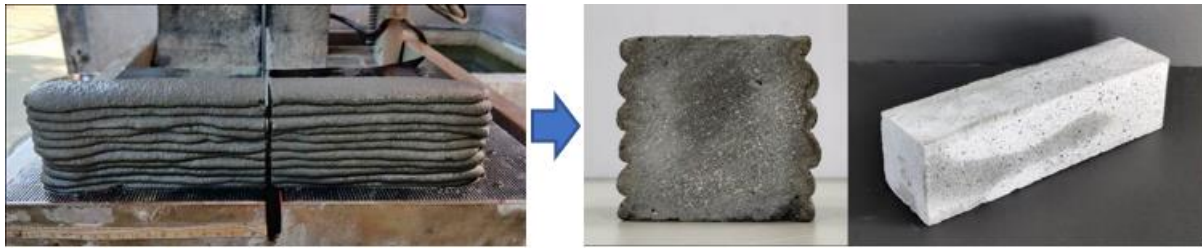
Figure 6. Preparation of printed specimens for compression and flexure testing
