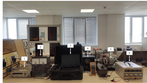
Fig. 5. Experimental setup for the standard squirrel cage induction motor: function generator (1), control unit of the magnetic powder brake (2), DAQ (3), magnetic powder brake (4), tested motor (5), and DC supply source (6).
