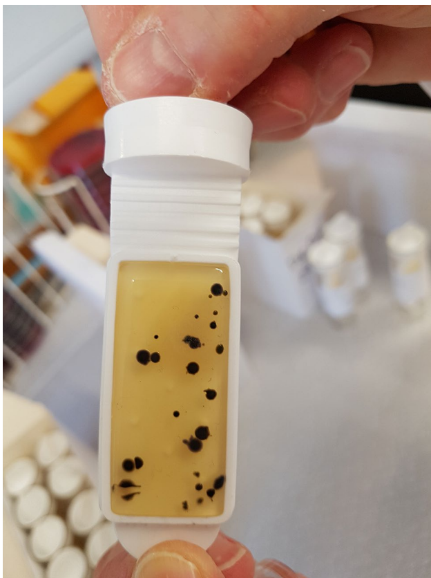
Fig. 2 Agar covered dipslide showing <5 cfu/cm 2
