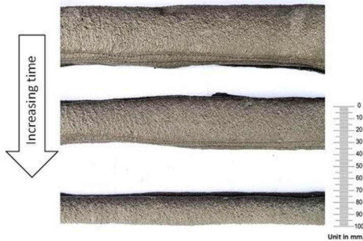
Fig. 6 Change of mortar width vs. time of plain mortar
