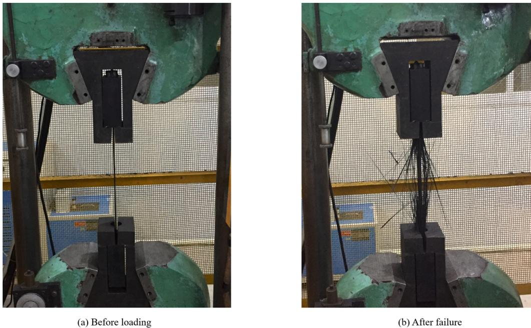
Fig. 6. Uniaxial loading tests for CFRP plates.
