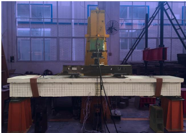
Fig. 7. Four-point bending test setup.
