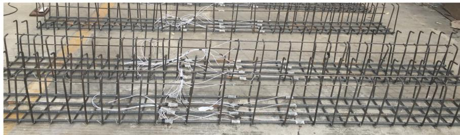
**Fig. 2.** Strain gauges attached on the bottom tensile reinforcements.
