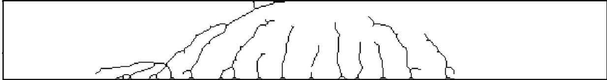
21 133 **Fig. 1** Typical crack pattern of an RC beam with fractal characteristics
