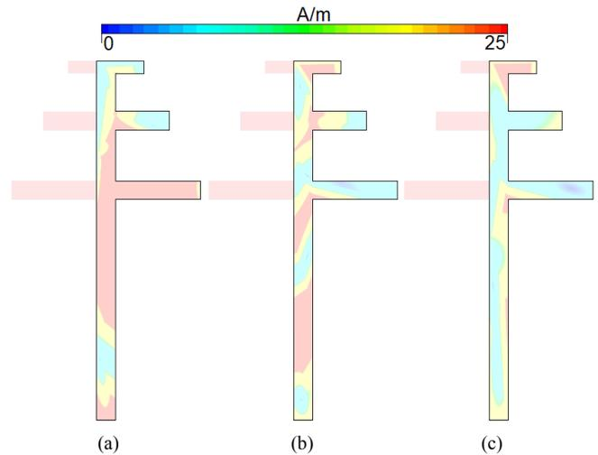
Fig. 3. Current densities at (a) 24, (b) 32, and (c) 65 GHz.
