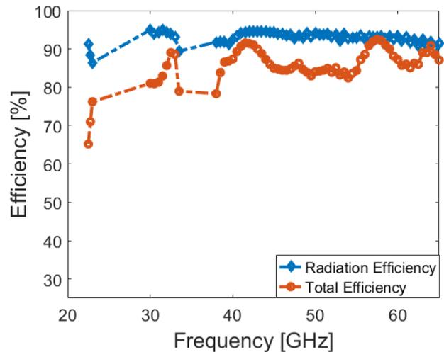
Fig. 4. Efficiencies of a single Yagi-dipole.
