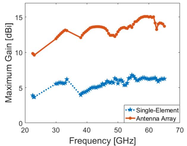
Fig. 6. Gains of the Yagi-element and its linear array configuration.
