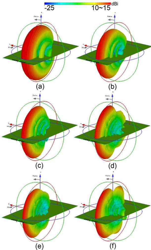
Fig. 5. Main radiations of the suggested super-wideband phased array at (a) 25, (b) 32, (c) 37, (d) 45, (e) 55, and (f) 65 GHz.
