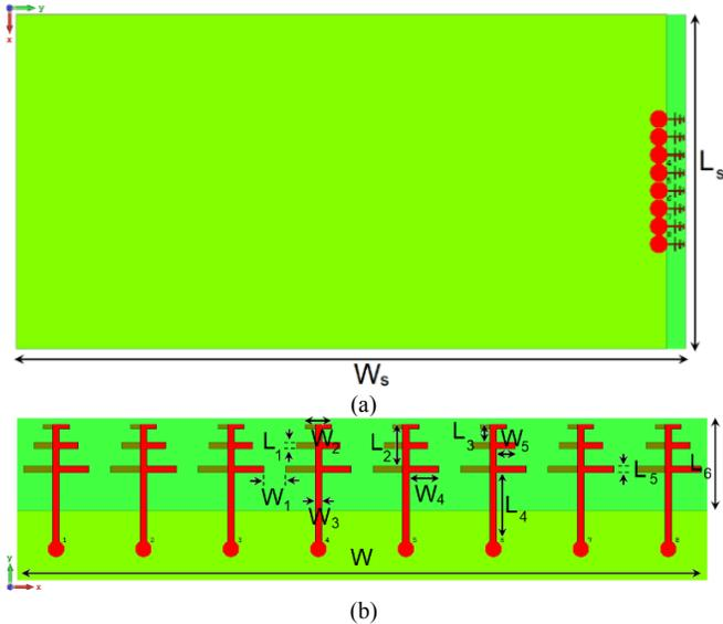
Fig. 1. (a) The suggested 5G mobile-phone antenna configuration and (b) its phased array schematic.
