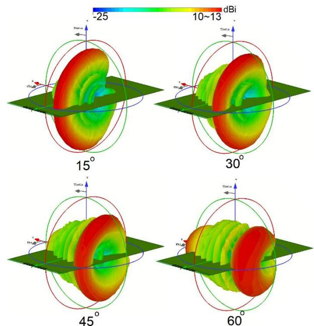
Fig. 7. 3D beam steering at 30 GHz.
