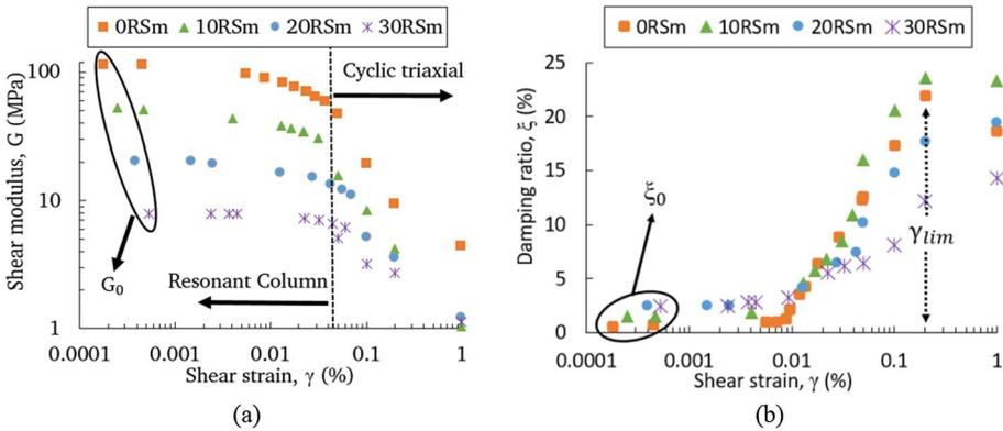
**Fig. 1** **a** Shear modulus and **b** damping ratio of RS<sub>m</sub> from small-to-large strains (Bernal-Sanchez 2020)
