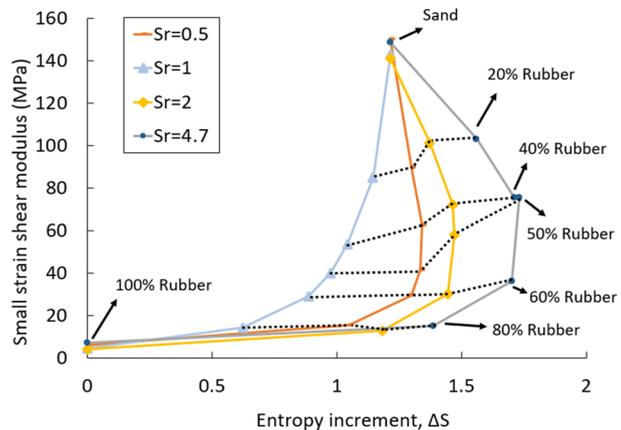
the shear stiffness is only dependant on the rubber content and the range of particle sizes retained in (limited) sieves.
