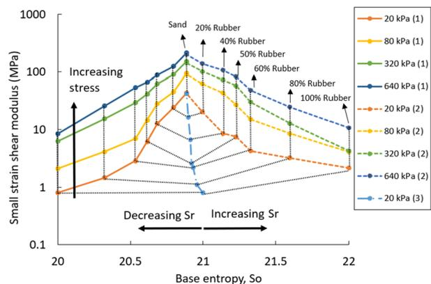
load-carrying chains are created amongst the small sand particles. However, this phenomenon is less appreciable at very large stress levels (i.e. 320 kPa and 640 kPa) and mixtures with both size ratios ( $S_r=0.5$  and 2) show relatively similar shear stiffness. This is attributed to the idea that rubber particles fully distort at such a high stress level and the development of the strength in the mixtures is mainly a result of the sand-to-sand contacts.
