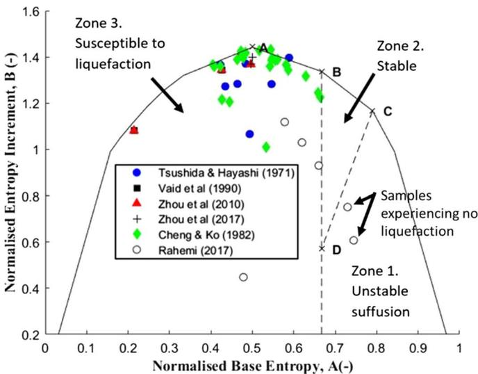
**Fig. 8** PSDs representing liquefaction susceptibility limits, as discussed by Barreto et al. (2019). Points A, B, C & D on a normalised entropy diagram are used to demonstrate regions of soil internal stability phenomena as proposed by Lőrincz (1986)
