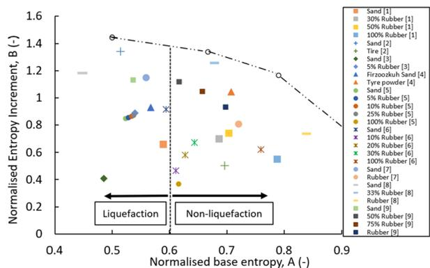
entropy coordinates are separated on the normalised entropy diagram in two regions related to the occurrence (or not) of liquefaction.
