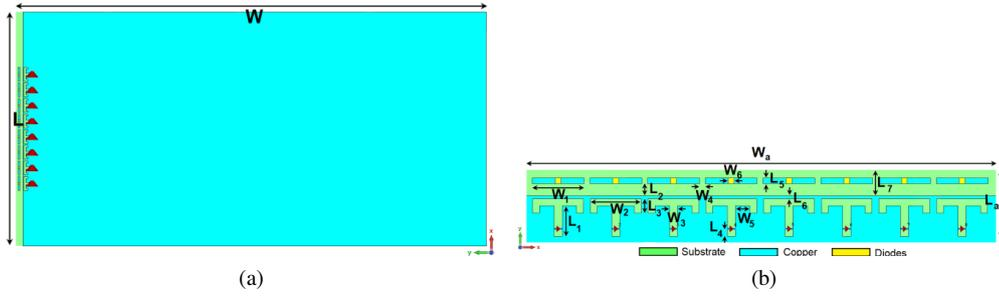
Figure 1: (a) The investigated antenna platform and (b) its linear array.
