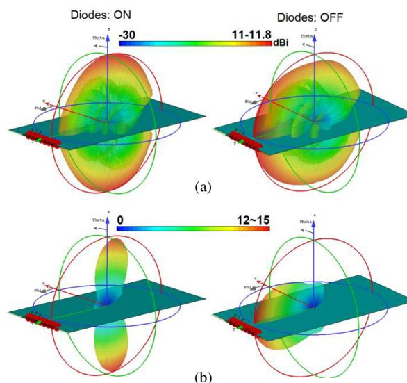
Figure 5: The results of radiation-mode reconfigurability for the smartphone array at 28 GHz (a) without and (b) with linear-scaling for a better view.
