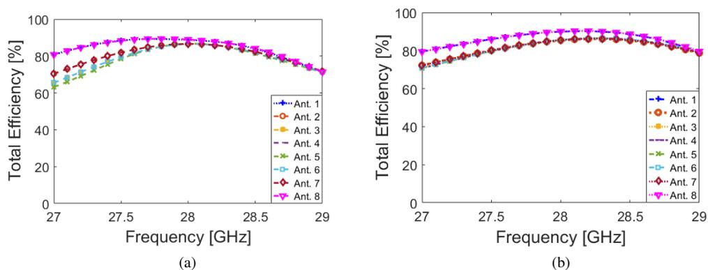
Figure 4: The results of antenna total efficiencies at 28 GHz for (a) diodes = ON and (b) diodes = OFF.
