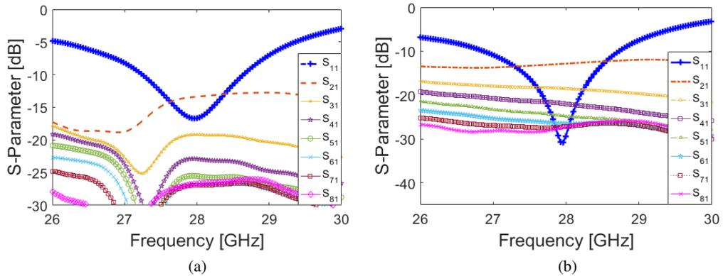
Figure 2: Simulated scattering parameters of the reconfigurable array for: (a) diodes: ON and (b) diodes: OFF.
