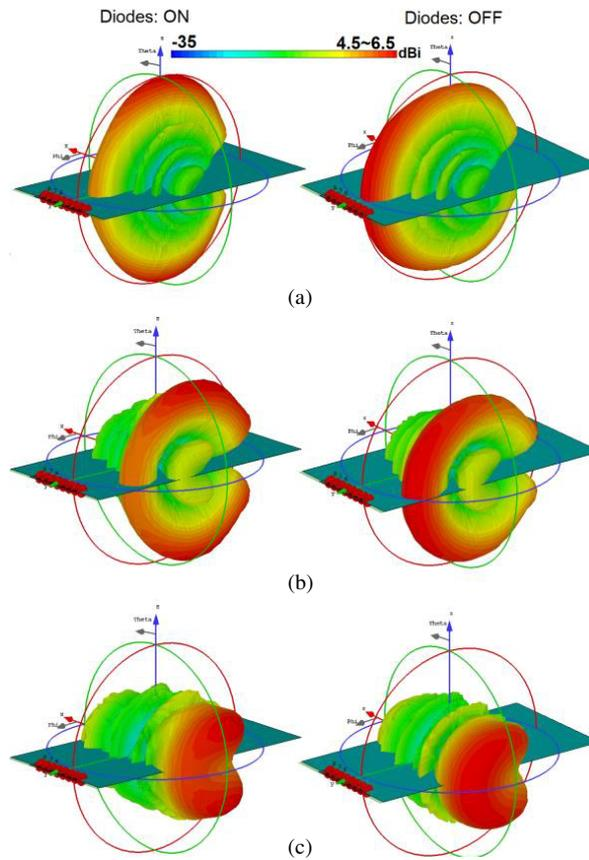
Figure 6: 3D beam-scanning at (a) 0, (b) 30, and (c) 60 degrees.
