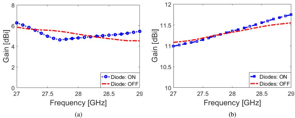
Figure 7: Maximum gain for the reconfigurable (a) single slot resonator and (b) its linear array configuration.
