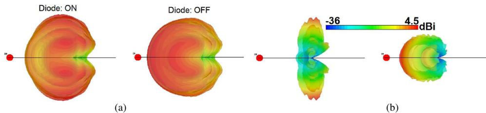
Figure 3: The results of radiation reconfigurability for the single-element antenna at 28 GHz (a) without and (b) with linear-scaling for a better view.
