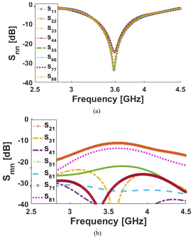
Fig. 2. (a)  $S_{nn}$  and (b)  $S_{mn}$  results for the studied MIMO antenna.
