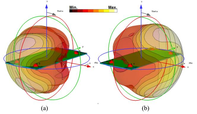
Fig. 3. Radiations of (a) first and (b) second resonators at 3.6 GHz.
