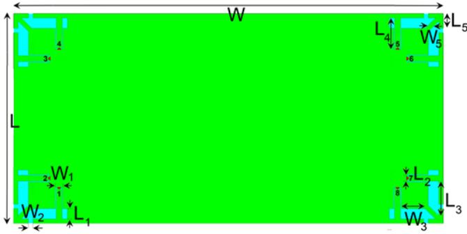
Fig. 1. Design details of the investigated MIMO smartphone antenna.
