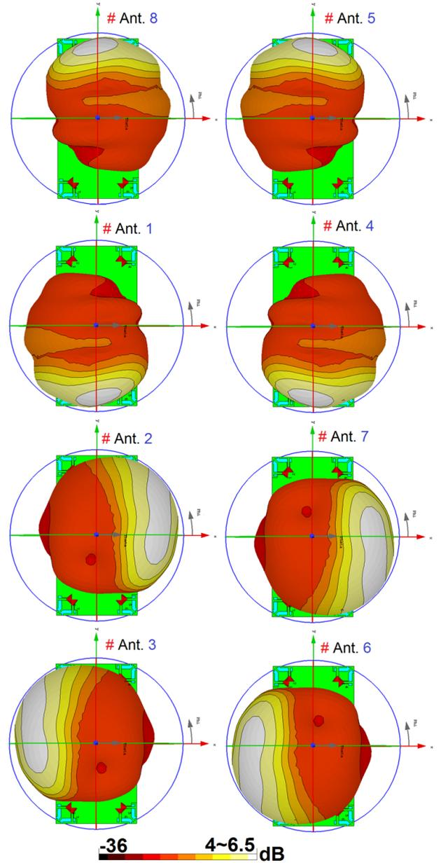
Fig. 4. Radiations of the CPW-fed diversity radiators at 3.6 GHz.
