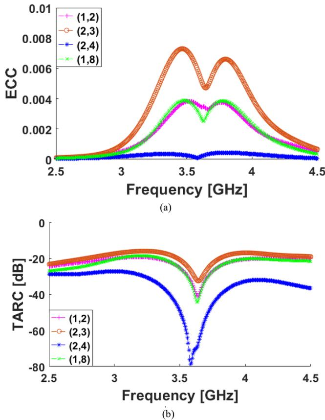
Fig. 5. (a) ECC and (b) TARC properties for the studied MIMO antenna.
