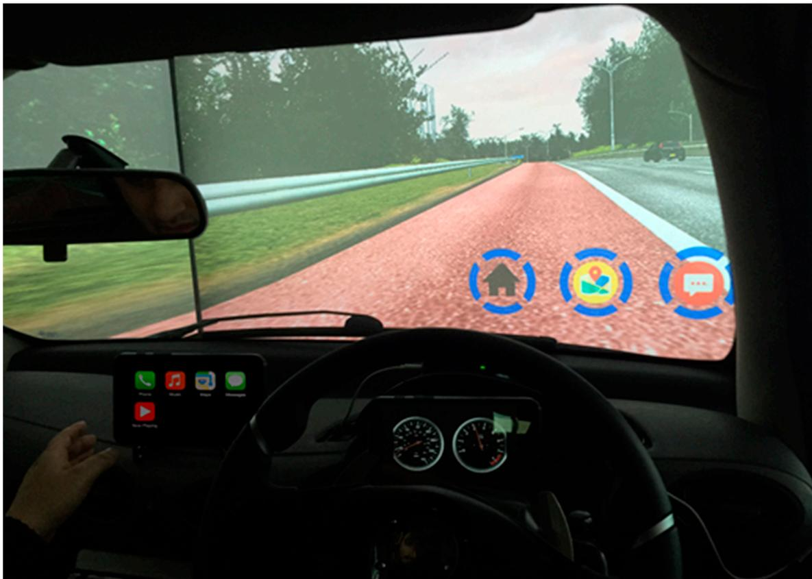
**Figure 1.** Screenshot of the fully functional Augmented Reality (AR) Head-Up Display (HUD) and conventional Head-Down Display (HDD) interfaces in the Virtual Reality (VR) driving simulator.
