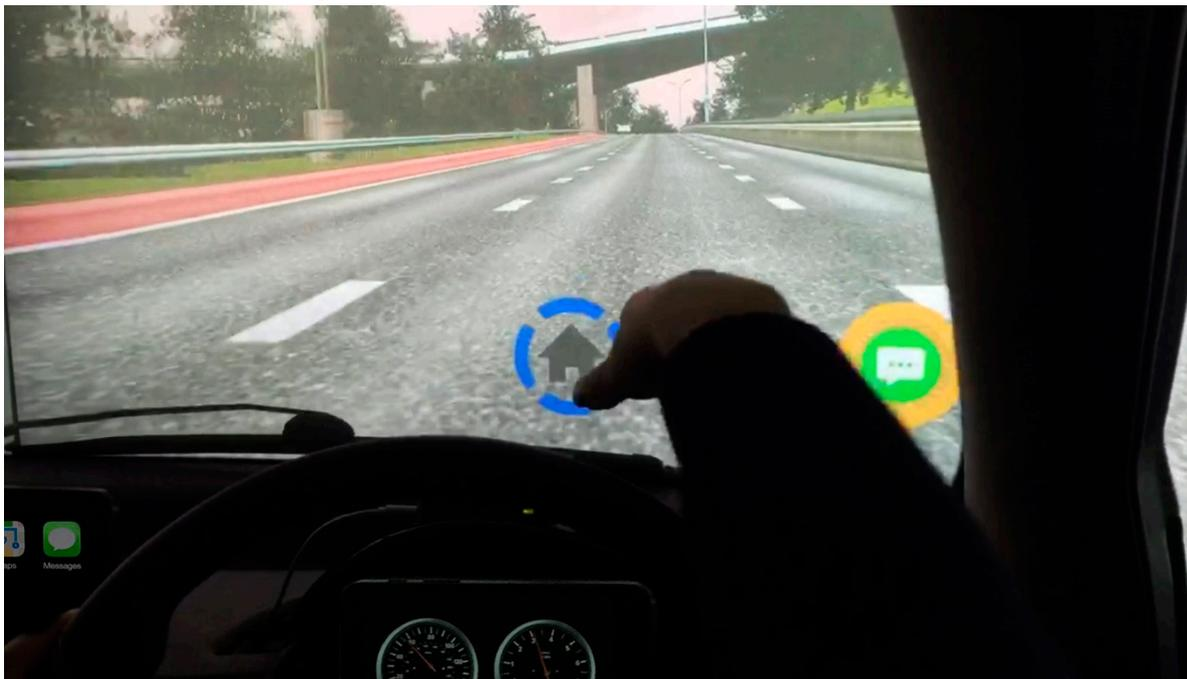
**Figure 2.** Screenshot of the fully functional AR HUD and conventional HDD interfaces in the VR driving simulator.
