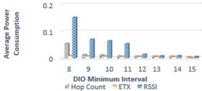
Figure 4-28. The Average Power Consumptions vs DIO Minimum Interval in mw
