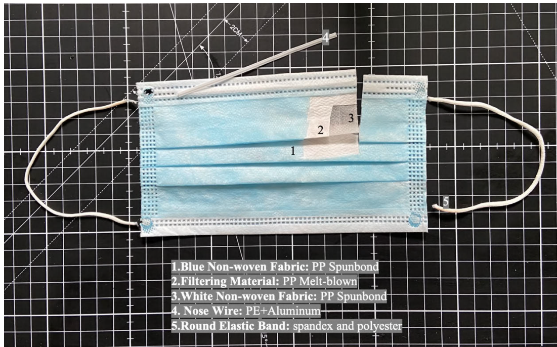
Figure 71. Composition of a facemask, Tao, 2021.
