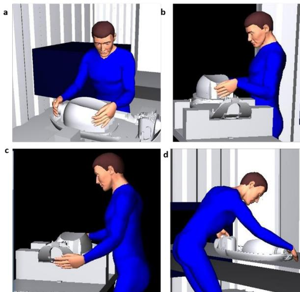
Fig. 3. (a) Positioning lamp on the jig; (b) Lifting lamp out of Support Beams; (c) Balancing product for placing into support; (d) lifting lamp from conveyor.
