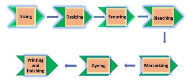
Figure 4. Various steps of wet textile processing.
