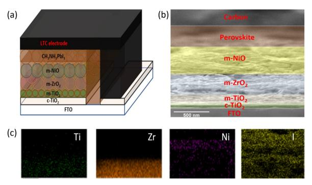
**Figure 6.** (a) Structural representation of LTCN device, (b) SEM image of LTCN device showing different layers, (c) EDX elemental analysis of Ti, Zr, Ni, I for the LTCN based device.
