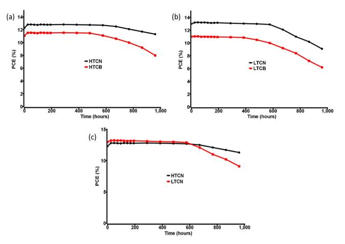
**Figure 8.** (a) Stability comparison between HTCN and HTCB devices, (b) stability comparison between LTCN and LTCB devices, (c) stability comparison between HTCN and LTCN devices.
