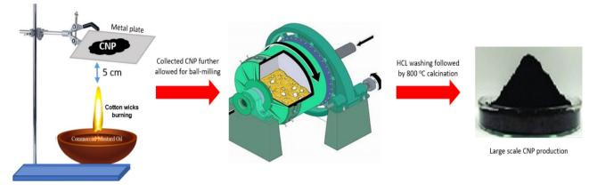
Figure 1. Schematic representation of carbon nanoparticles synthesis utilizing burnt cotton wicks.
