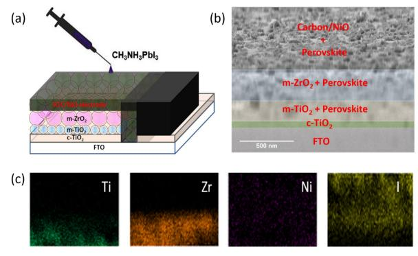
**Figure 4.** (a) Structural representation of HTCN device, (b) SEM image of HTCN device showing different layers, (c) EDX elemental analysis of Ti, Zr, Ni, I for the HTCN based device.
