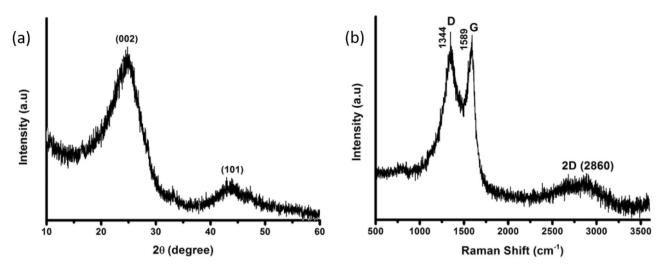
Figure 2. (a) XRD pattern of as-synthesized CNP, (b) respective Raman spectrum.
