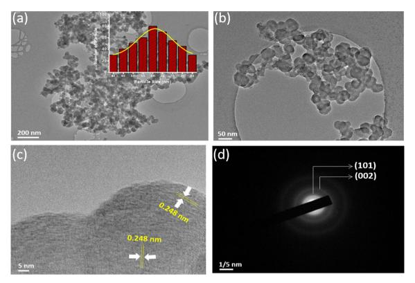
**Figure 3.** (a) and (b) TEM bright field images of synthesized CNPs at different magnification (inset: corresponding particle size histogram), respectively, (c) HRTEM image of single CNP nanoparticle, (d) SAED pattern of CNP.
