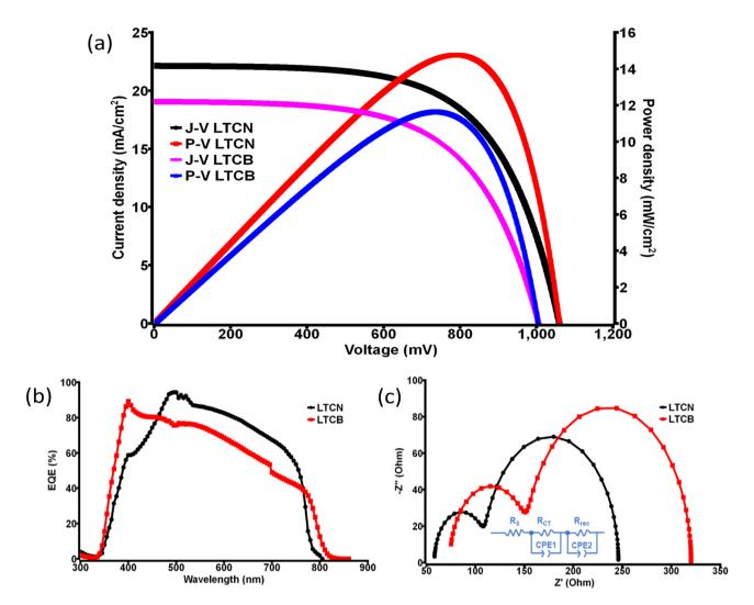
**Figure 7.** (a) J–V and P–V curves of the champion LTCN and LTCB devices, (b) EQE of the champion LTCN and LTCB devices, (c) EIS representation of the champion LTCN and LTCB devices along with the electrical circuit diagrams.
