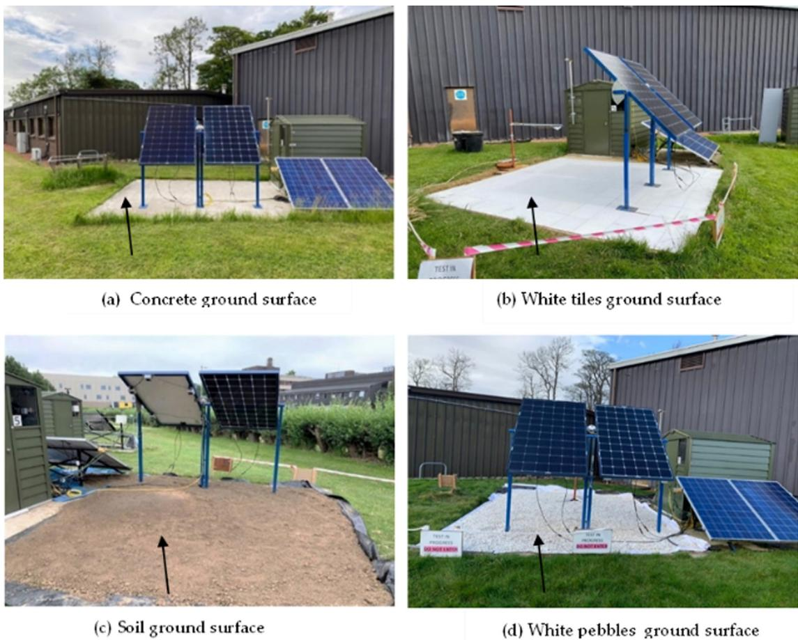
Fig. 3. (a) Concrete (b) White tiles, (c) Soil and (d) White pebbles ground surface
