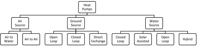
Fig. 9. Heat pump types.
