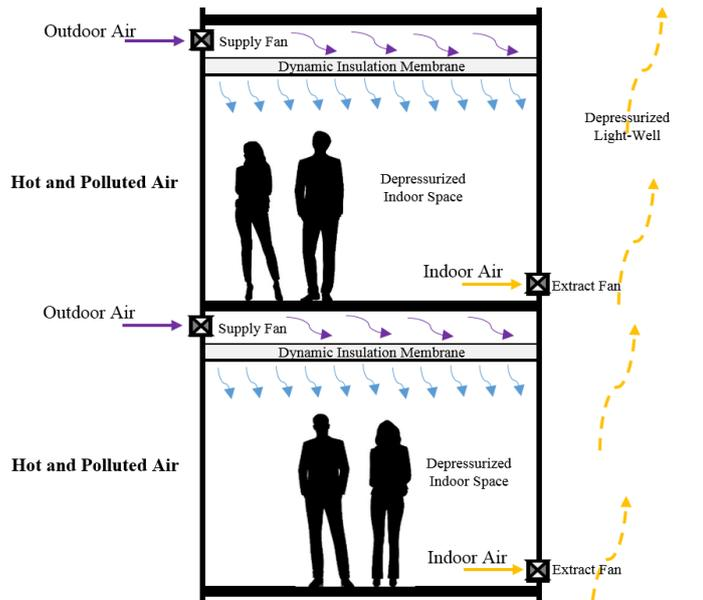
FIGURE 1: Schematic design concept of the Airhouse system (Image by the Author)
