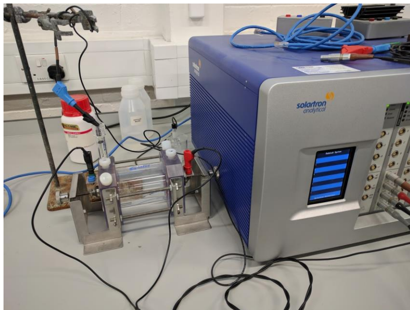
Figure 39: EIS experimental set-up using Gamry Paracell and Solartron Analytical Modulab.
