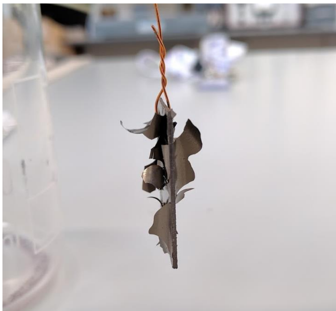
Figure 52: Severe delamination of nickel coating from substrate.
