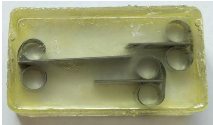
Figure 31: Cross-sections prepared in epoxy resin.
