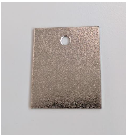
Figure 36: High quality NiP/gelatine composite coating produced with ultrasonically processed microgels. Coupon dimension = 25 mm x 30 mm.
