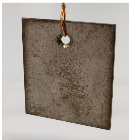
Figure 34: NiP/gelatine composite coating with reduced deposit thickness at edges. Coupon dimensions = 25 mm x 30 mm.
