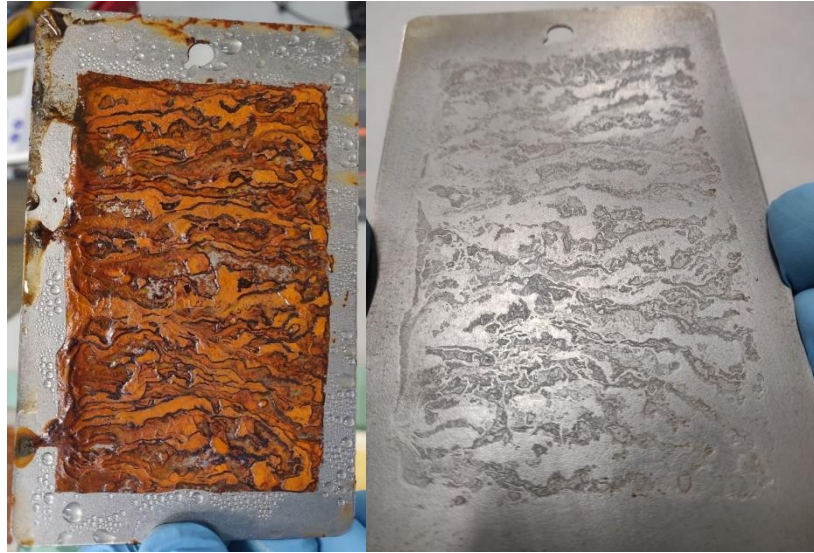
Figure 37: Plain mild steel S-35 Q-Panel used to confirm corrosion rate of cabinet. Area of corrosion = 60 mm x 100 mm.
