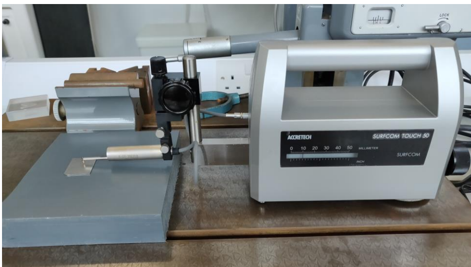
Figure 41: Surfcom Touch 50 performing coating roughness measurements on uncoated reference sample for comparison with NiP/gelatine composite coatings.
