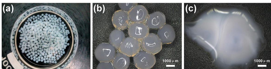
Figure 22: a) Ag-alg capsules, b) Optical image of Ag-alg capsules, c) The Ag-alginate capsule that disintegrated when exposed to chloride ions [57].
