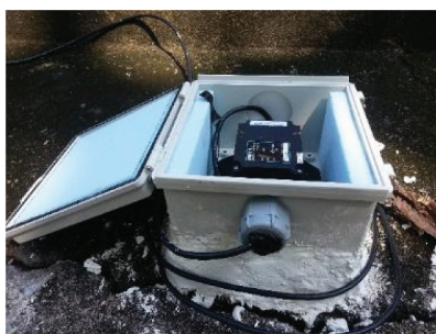
Figure 2. Specification and installation of accelerometer.
