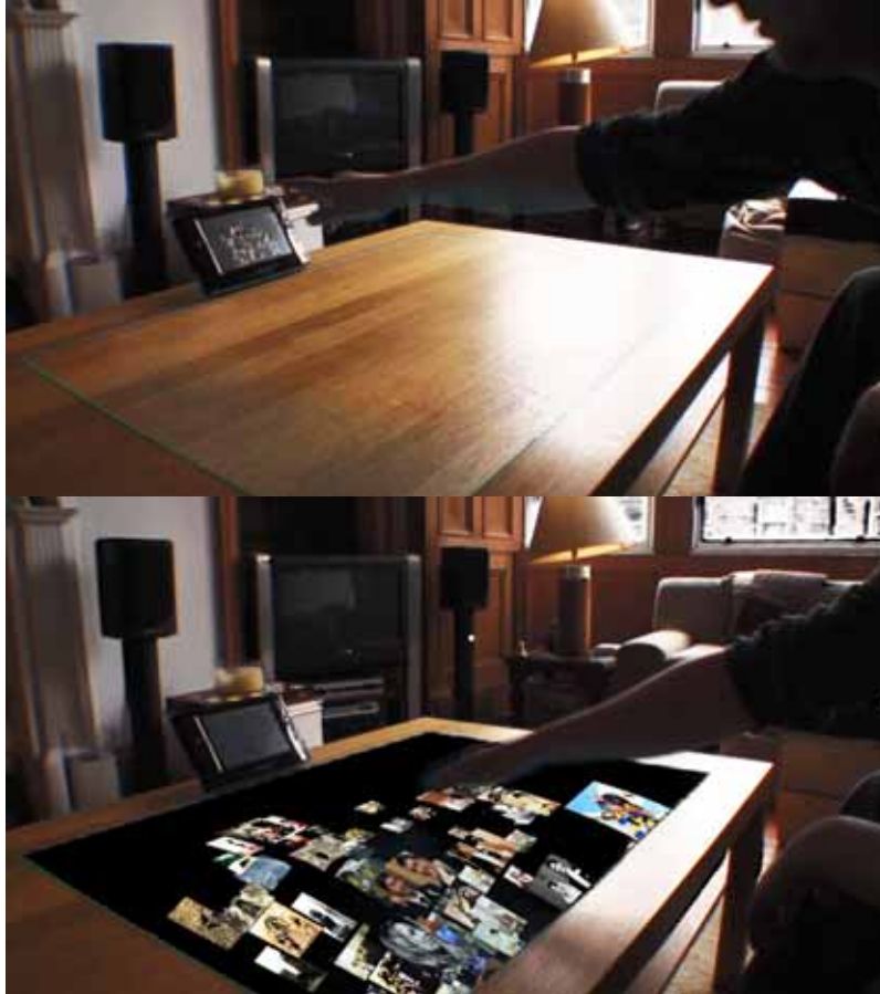
Figure 16. An example of a multimodal interaction moving between displays from a digital photoframe to a smart coffee table.
