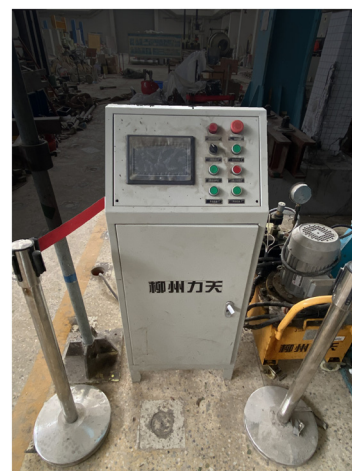
Figure 4: Hydraulic control system.
