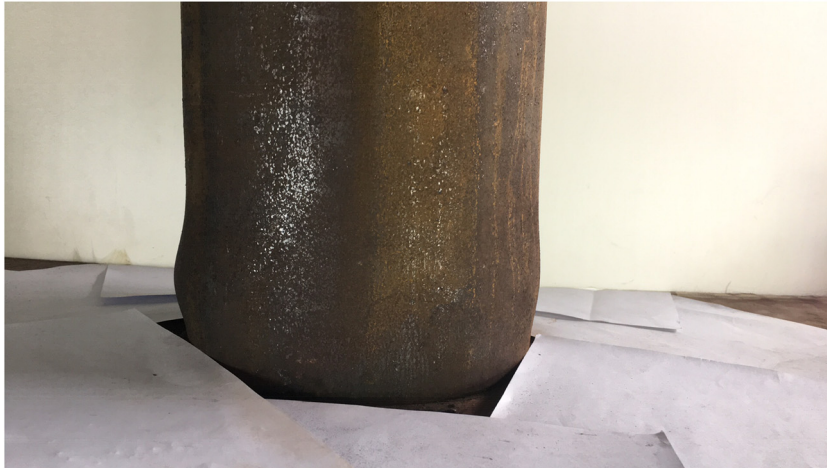
Figure 6: Typical failure mode of test piece.
