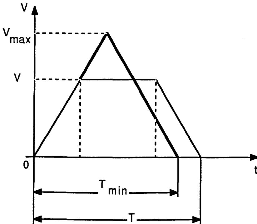
Fig. 3.2 Optimum velocity-time graph.
