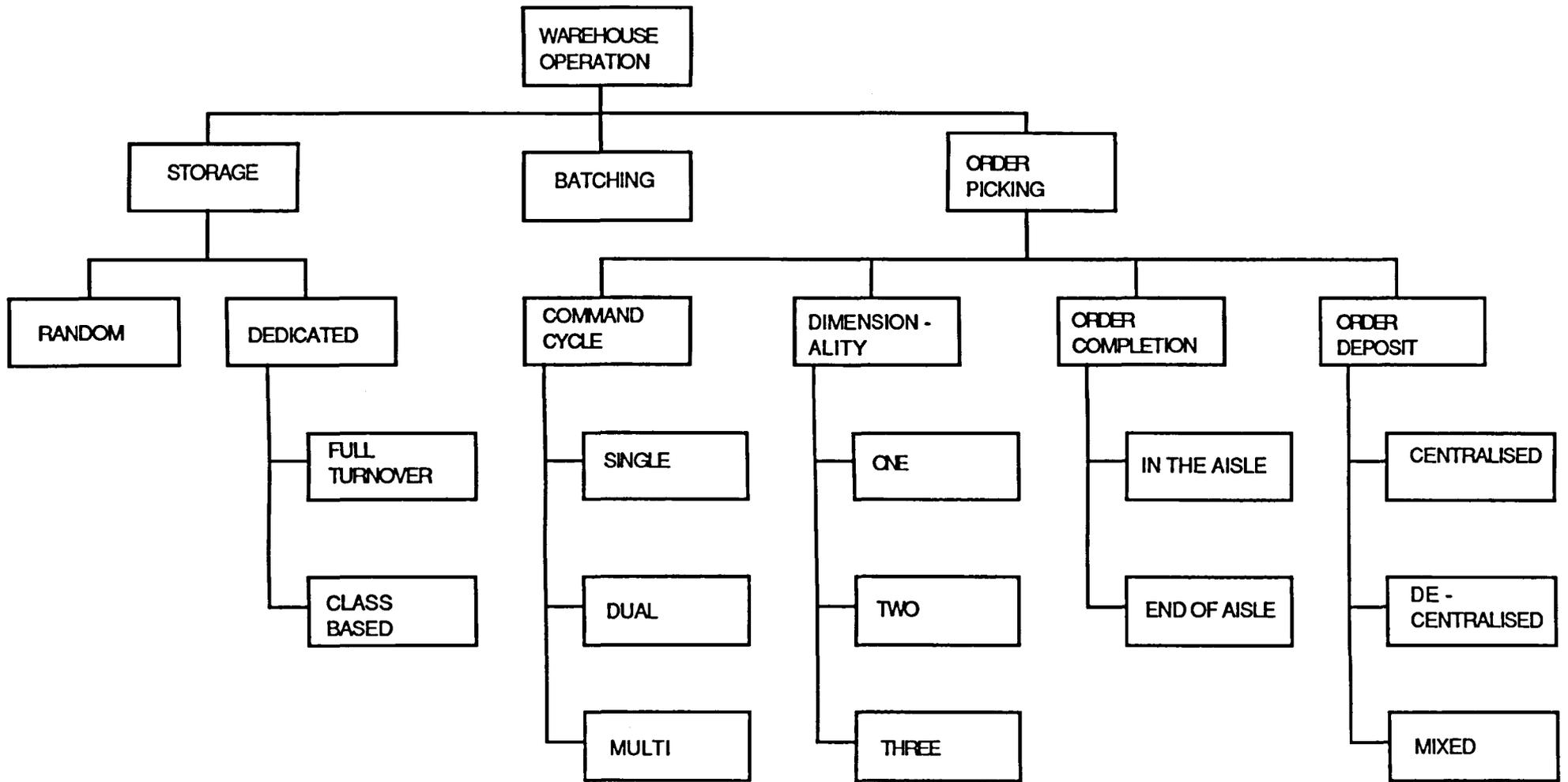
Fig. 1.1 Classification of warehouse operation related to storage and retrieval
