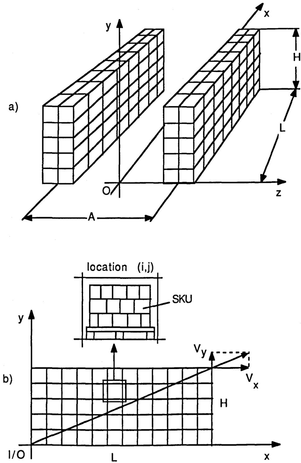
Fig.1.2 An aisle in a high bay warehouse; a) pictorial view; b) front view of a rack
