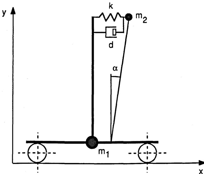
Fig. 3.1 Two mass equivalent model of a stacker crane
