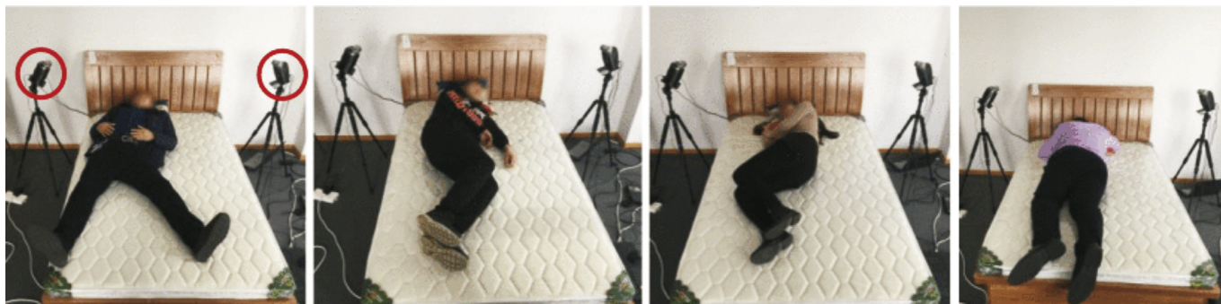
Fig. 4. Experimental setup to monitor abnormal respiratory using ultrasound signals (reprinted from Ref. [99] with permission).
