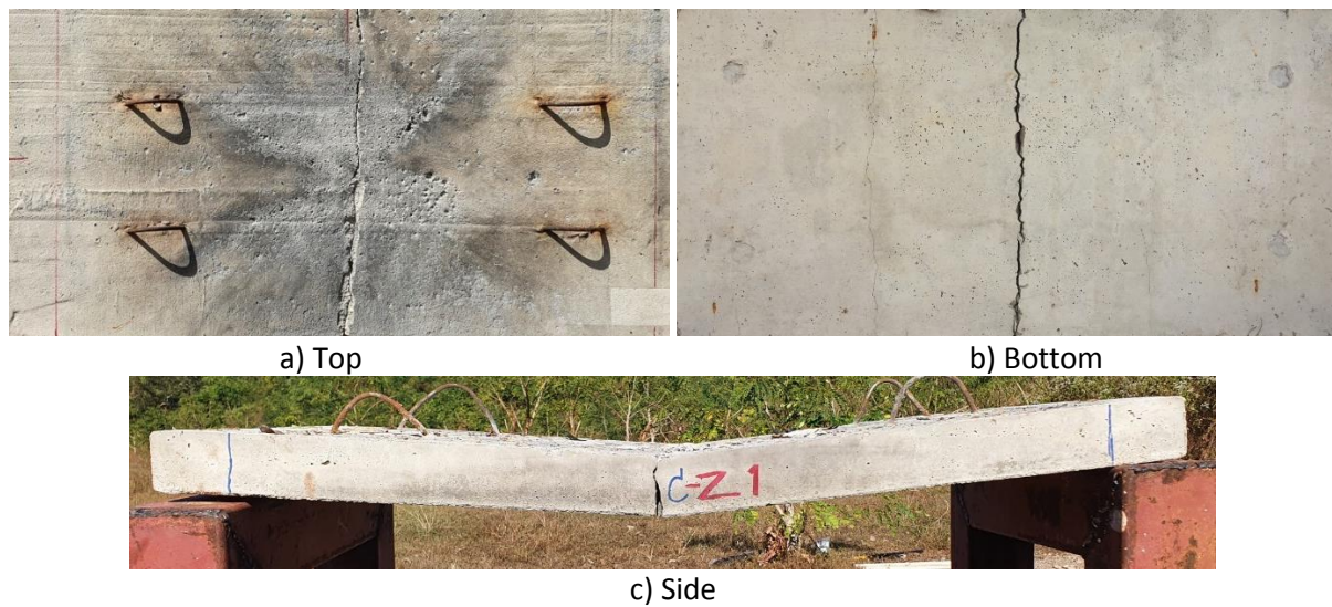
40 41 42 43 44 45 46 47 48 49 50 51 52 53 54 55 56 57 58 59 60 61 62 63 64 65 Figure 12. Complete flexural failure pattern
