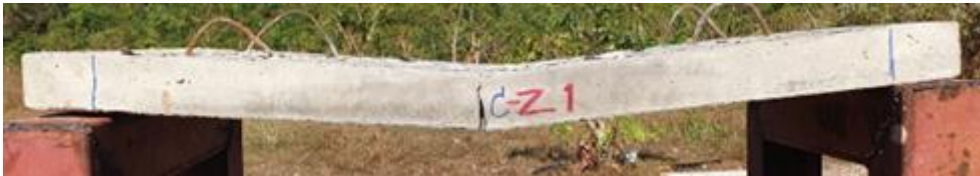
Figure 12c. Complete flexural failure pattern
