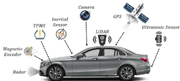
Fig. 1 Commonly used sensors in smart vehicles
