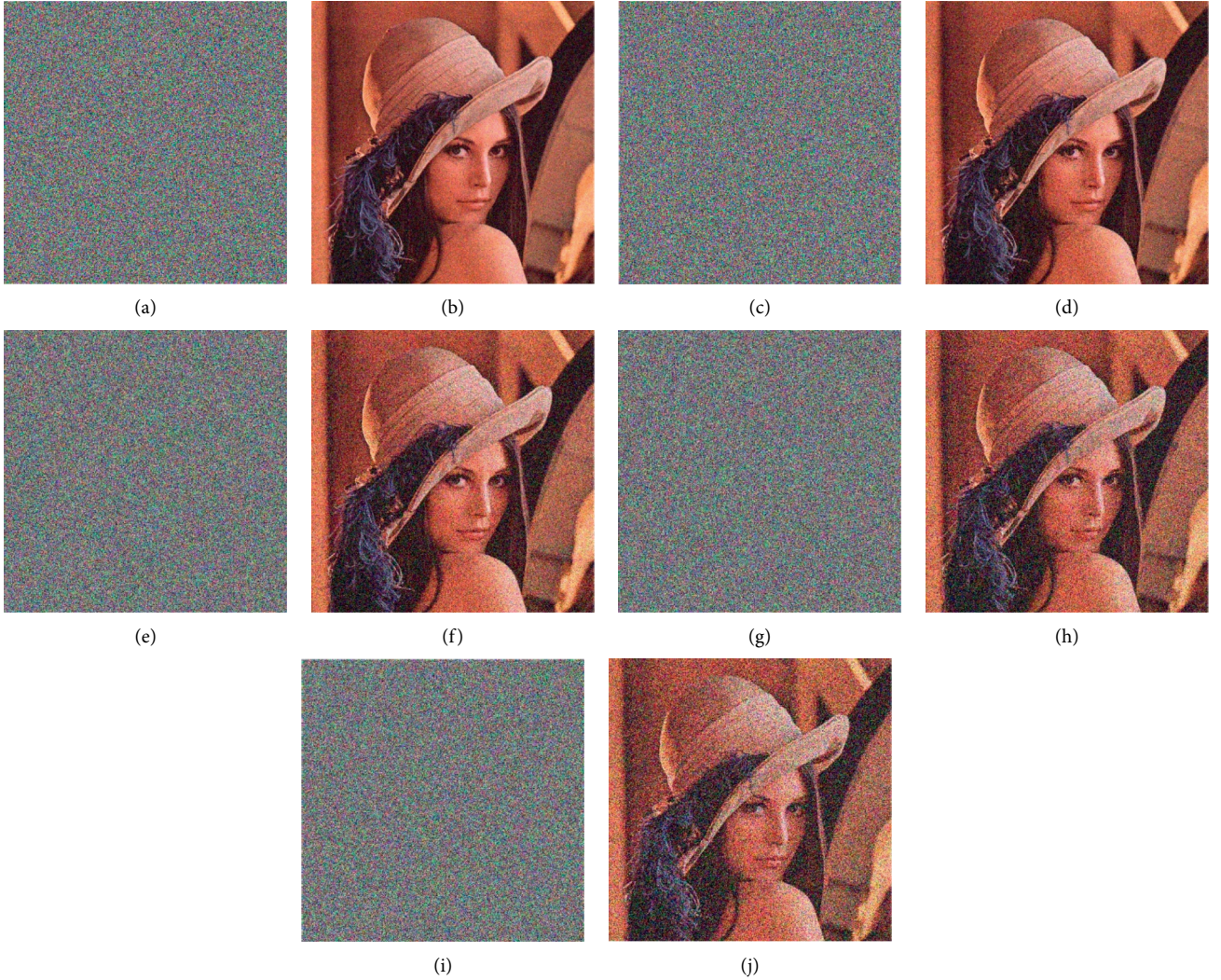
FIGURE 8: Data loss and noise attacks on encrypted images. (a) The untouched encrypted image and (b) its decrypted image; (c) the encrypted image with 3 \times 3 data block loss and (d) its decrypted image; (e) the encrypted image with 9 \times 9 data block loss and (f) its decrypted image; (g) the encrypted image deteriorated with 0.005% Salt and Pepper noise and (h) its decrypted image; (i) the encrypted image deteriorated with 0.02% Salt and Pepper noise and (j) its decrypted image.
