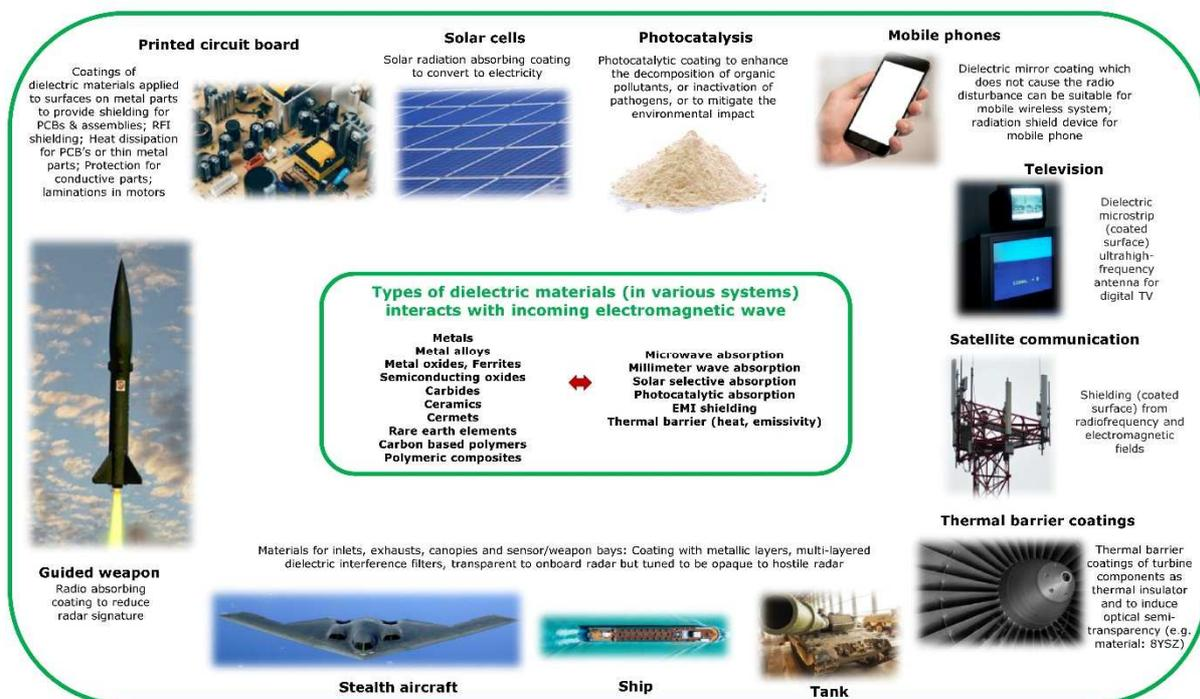
**Fig. 1.** Example applications of dielectric material that can interact with EM waves, and how their manufacture using coating techniques can address the technological requirements.
