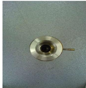
**Figure 3b** Membrane core holder without seal
