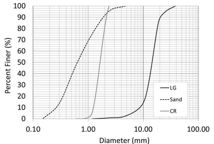
Fig. 1. Grading curve of aggregates.
