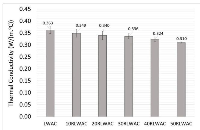
Fig. 4. Thermal conductivity (λ) of LWAC and RLWAC.
