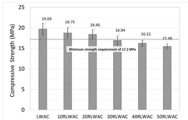
Fig. 3. Compressive strength of LWAC and RLWAC.
