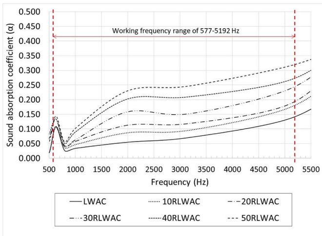
Fig. 5. Sound absorption coefficient ( $\alpha$ ) of LWAC and RLWAC within working frequency range.
