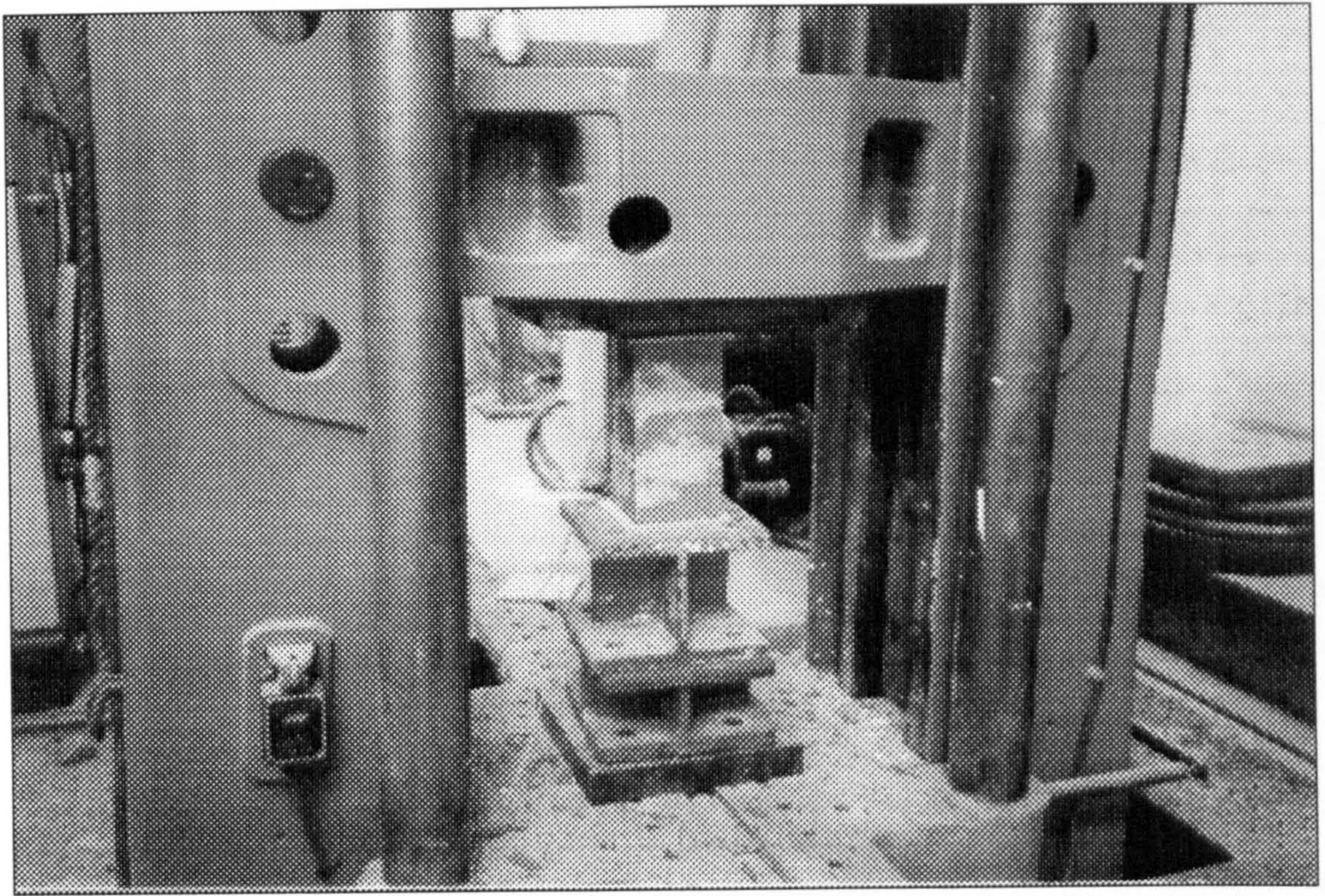
Figure 5.1 The Avery Denison hydraulic testing rig
