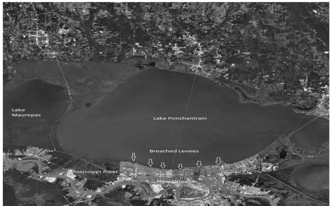
Figure 2.10 Image showing the breached levees in New Orleans during Hurricane Katrina [source:(Google Earth)]
