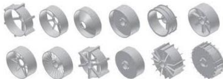
Figure 1. Typical rotor and stator structures [12]
