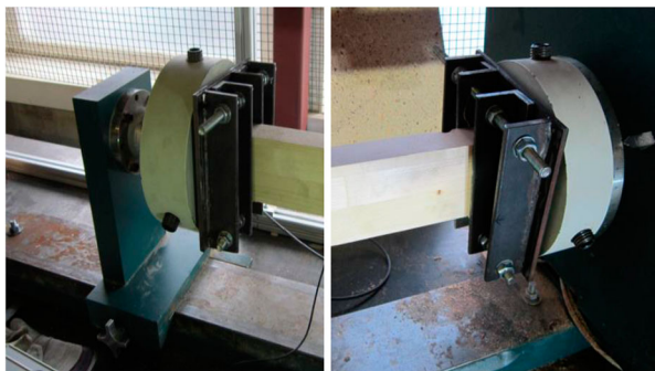
Figure 4. Clamps of the torsion tester at the fixed end (left) and at the rotating end (right).
