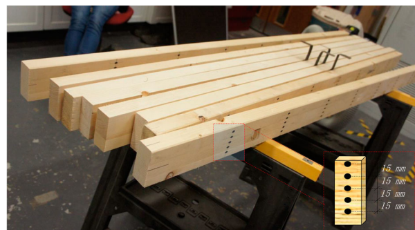
Figure 2. Torsion specimens after applying targets to their surfaces.
