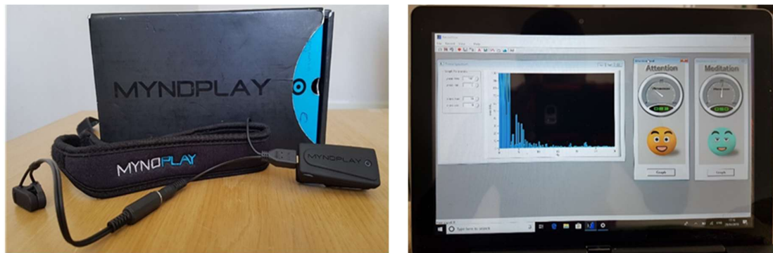
Figure 3-4: The NeuroSky Mobile MindSet (MYNDPLAY) and the display screen on Windows tablet during EEG data collection
