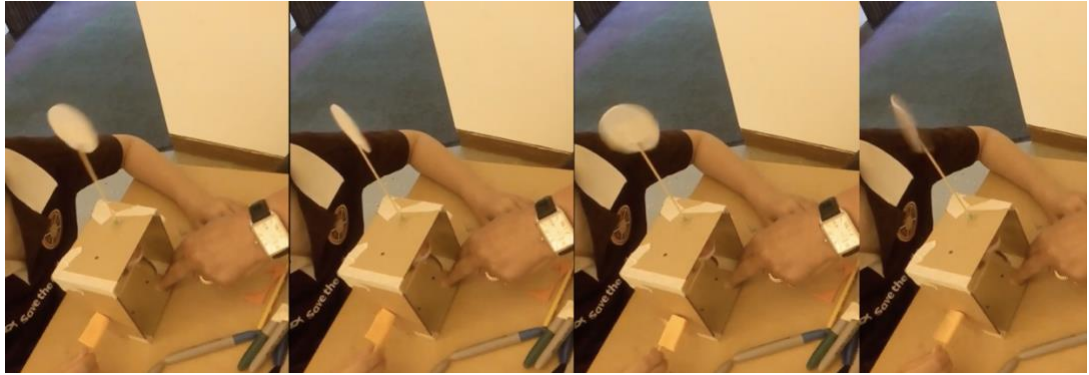
Figure 57: Football automaton (P2_D3) using an eccentric circular cam
