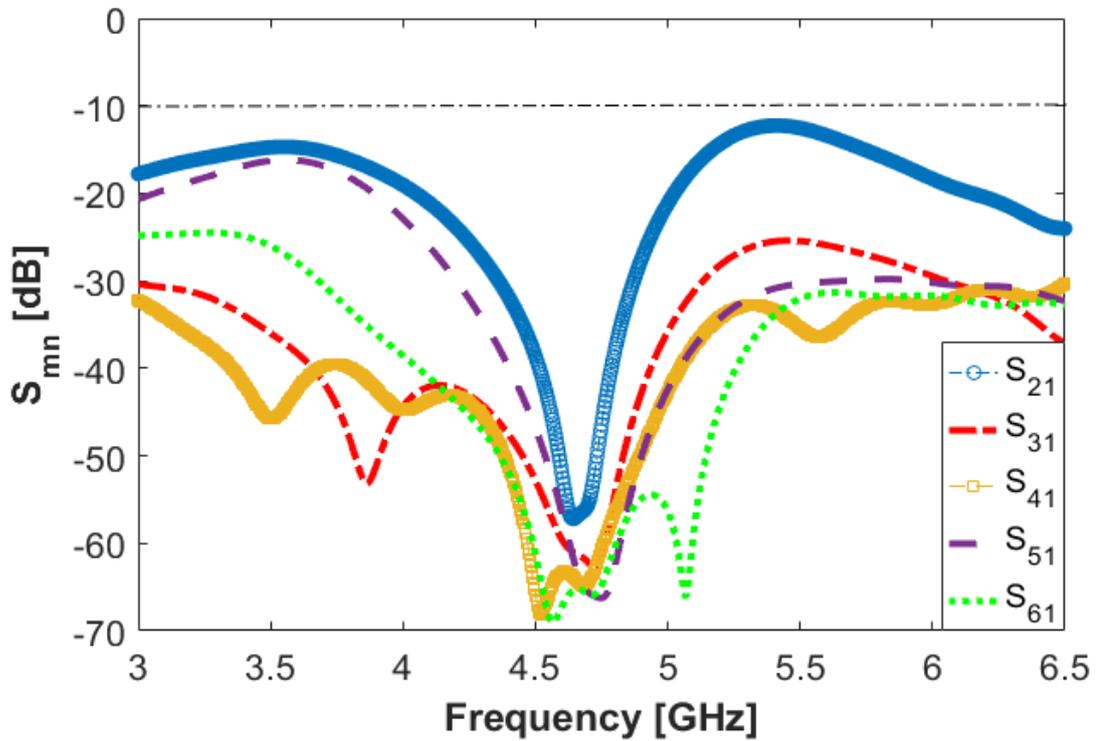
Fig. 4. Simulated mutual coupling results ( $S_{mn}$ ) of the MIMO antenna array.
