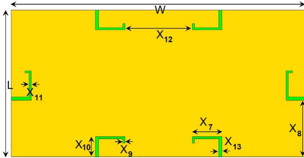
Fig.2. Bottom View of Schematic structure of the designed MIMO smartphone antenna
