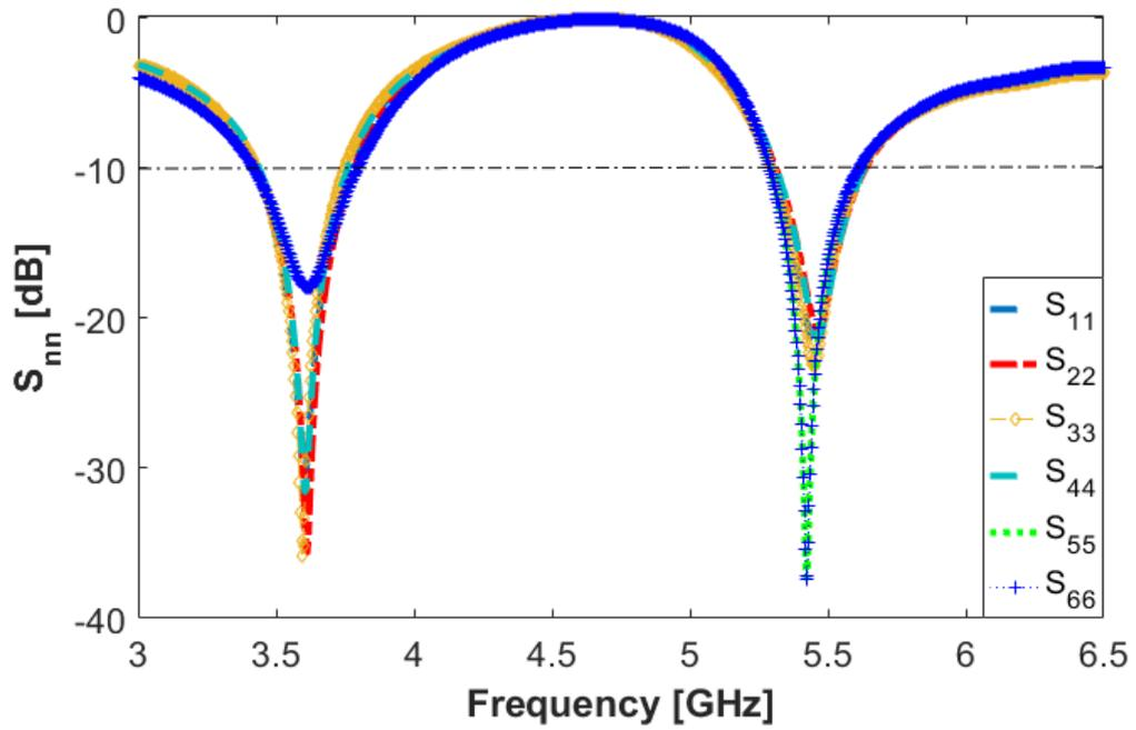
Fig. 3. Simulated return loss ( $S_{nn}$ ) of the MIMO antenna array.
