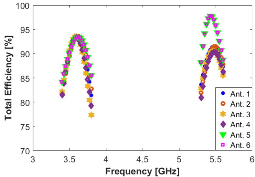
Fig. 8. Total efficiencies of the MIMO antenna over its operation band.
