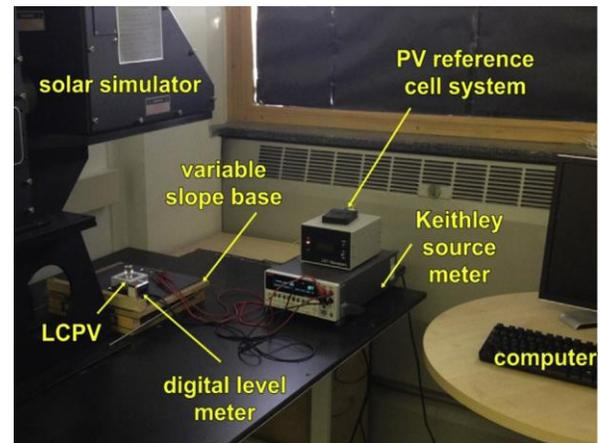
Fig. 2. Indoor experimental setup for RTP-PV characterization.
