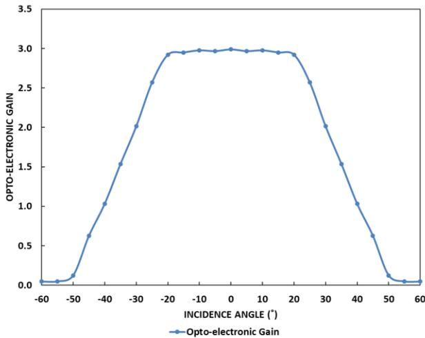
Fig. 5. The angular response of the RTP-PV device.
