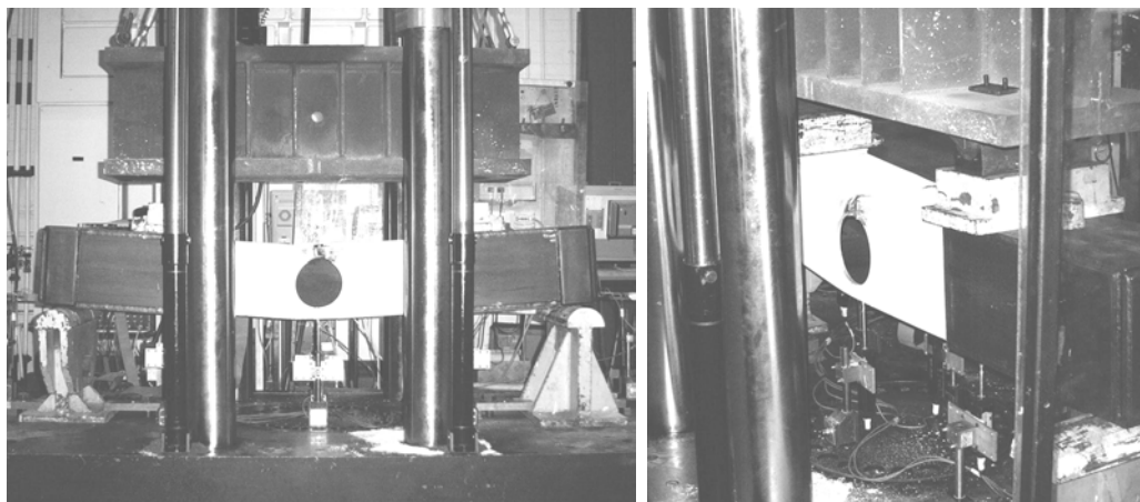
Figure 3-2: The four-point loading test apparatus
