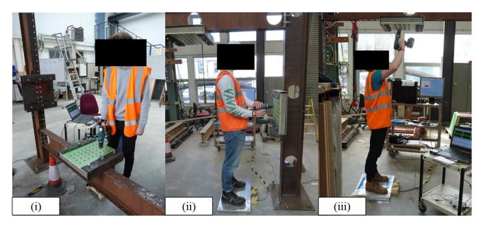
Figure 2. Test postures (i) vertical downwards similar to ISO 28527-5 posture, (ii) horizontal and (iii) vertical overhead.
