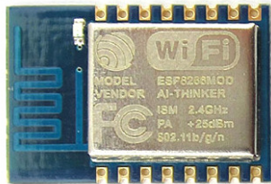
Figure 3: ESP8266 (dimensions: 16 x 24 mm)
