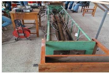
a) Installation of CFRP rods.
