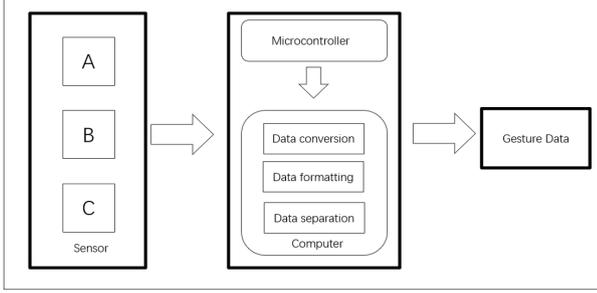
Figure 7: Data acquisition process
