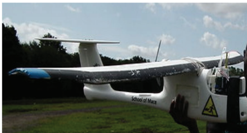
Figure 3. A picture of the integrated ozonesonde and Skywalker airframe at the Hough End Fields site.
